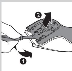
**4** Tilt the handle of the screwdriver downwards (1) and separate the back panel from the appliance (2).
